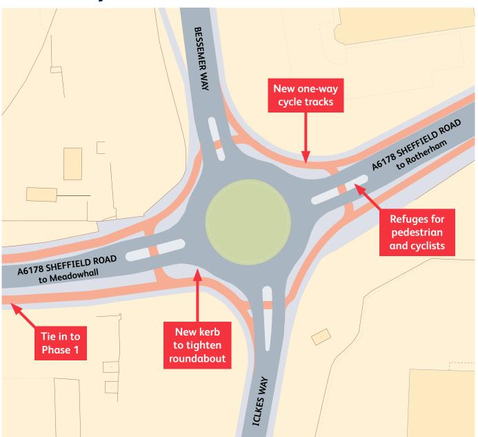
The carriageway approaches to this roundabout will be made narrower to:
