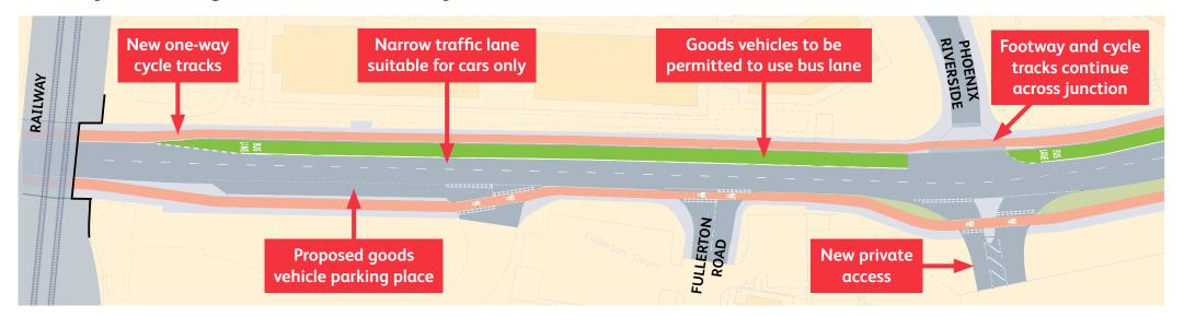
One-way cycle tracks are proposed on each side of the road, which will continue with priority across side roads and accesses; all side roads and accesses will remain open. We intend to reconstruct the side road entry at Phoenix Riverside so that footway and cycle tracks continue at same level across the side road (similar to at a driveway).
