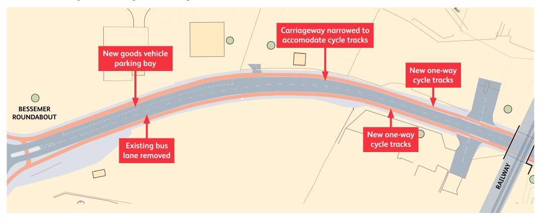
The proposed design for this section of the scheme is one-way cycle tracks on each side of the road, separate from and at different level to the adjacent footways; the carriageway will be narrowed to accommodate these.
