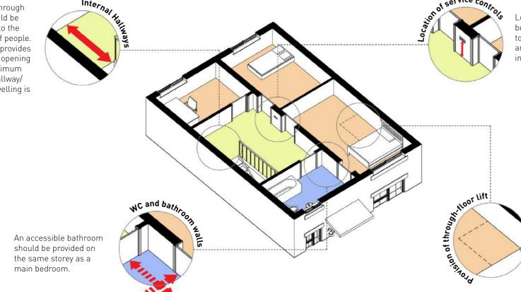
Location of service controls should be within a height band of 450mm to 1200mm from the floor level and at least 300mm away from any internal room corner.
