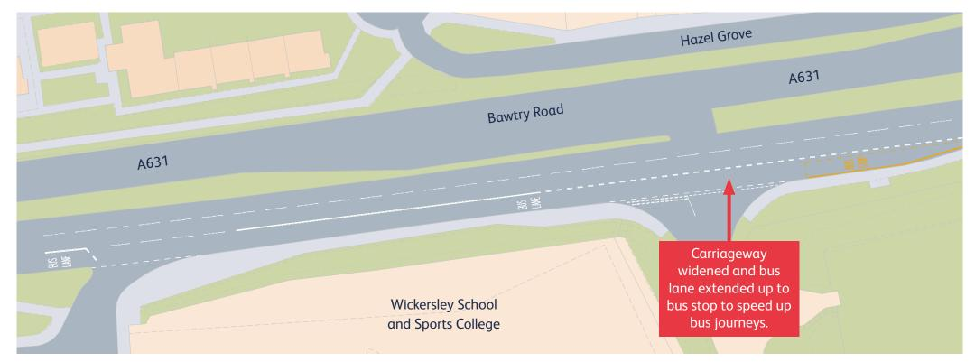
An additional carriageway will be constructed to join up the existing bus lane at Wickersley School with the existing bus stop lay-by upstream of the access to the water works. This is intended to allow buses to proceed from that bus stop without having to emerge into the main flow of traffic.
