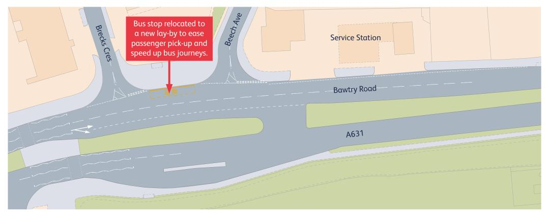
It is proposed to remove the existing service road between Brecks Crescent and Beech Avenue. The existing bus stop will be located to a new lay-by, immediately adjacent to the main carriageway. This will make it easier for bus drivers to see whether there is anyone waiting to board at the stop, and will improve the ease at which bus drivers can emerge back onto the main carriageway.
