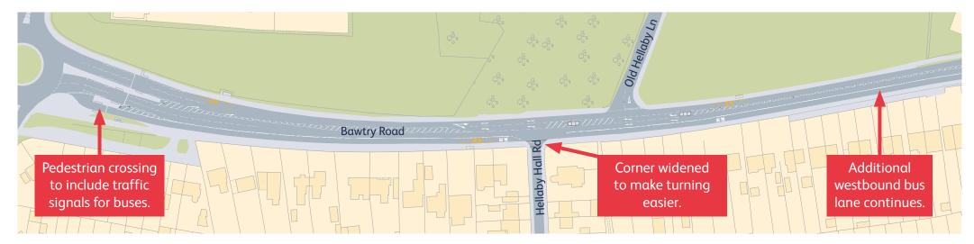
The existing pedestrian crossing on the eastern arm of Denby Way Roundabout will be amended to provide a set of bus-presignals, to allow buses to rejoin the main carriageway.
