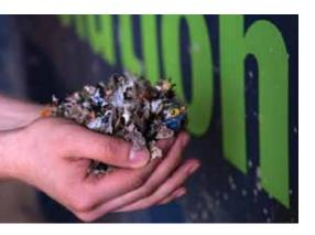
The smallest waste produced from the MBT plant is called 'fines'. This is transferred under cover to the AD building next door, where it is fermented for four weeks. This produces methane gas which will be used to generate electricity to supply the Bolton Road site with the surplus being sold to the National Grid.
