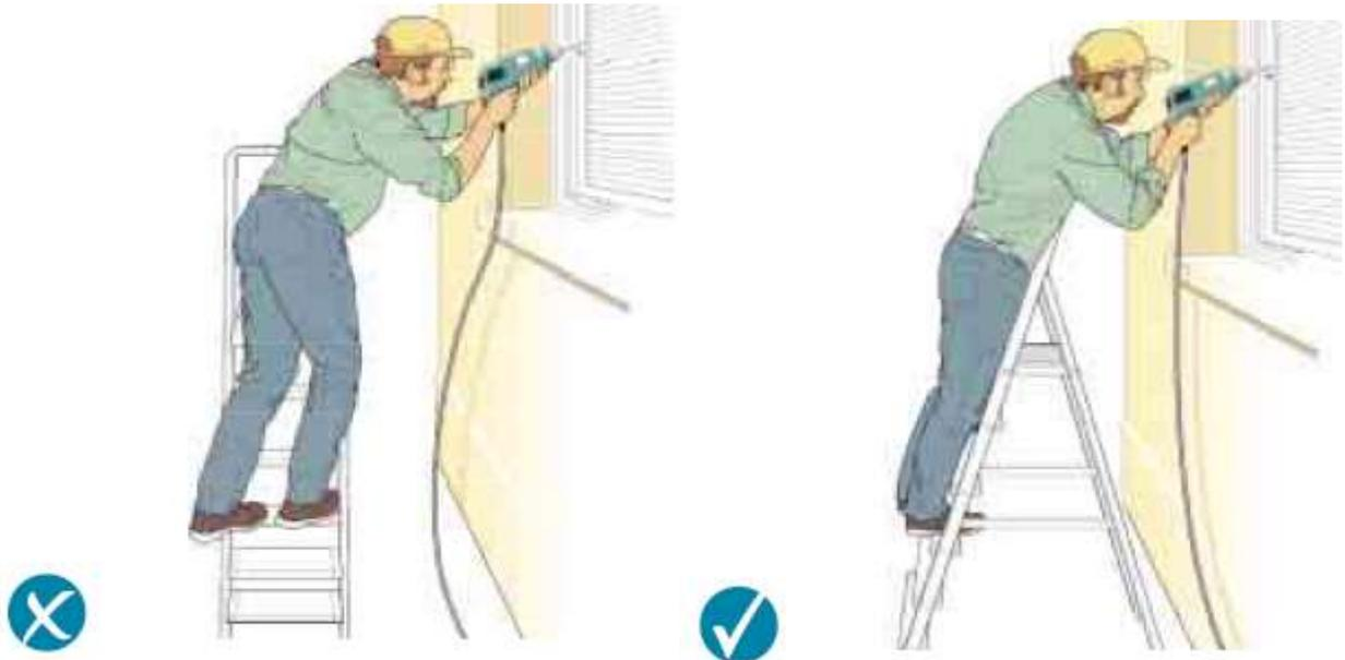
Figure 2a **Incorrect** - steps side-on to work activity
