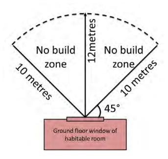
15 Setting an extension away from a habitable room window will reduce any potential loss of daylight and appear less overbearing to the neighbour.
