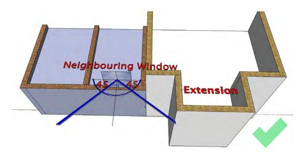
A rear extension close to a neighbour's habitable room can create an unacceptable loss of daylight and create an oppressive overbearing impact.
