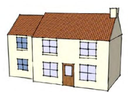
Appropriate subservient extension set back with a lower roof line
